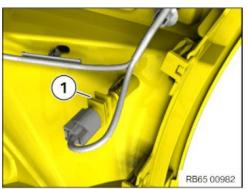
• Clip in temperature sensor (1) into the bumper panel.
