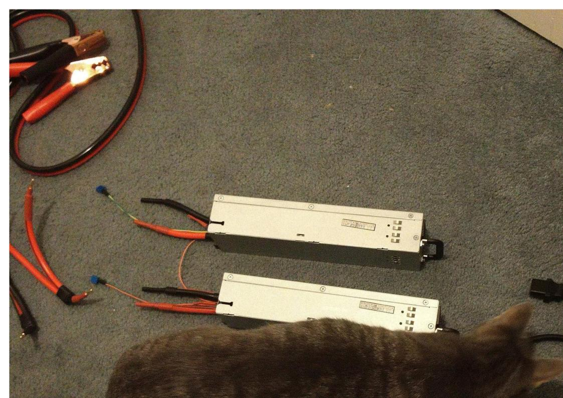
My PSUs were set to 13.5v and I think I was losing voltage due to the resistance of the long jumper cables and my crappy soldering. The car's battery terminals were reading 13.30v on my multimeter during flashing and did not budge the whole time.
