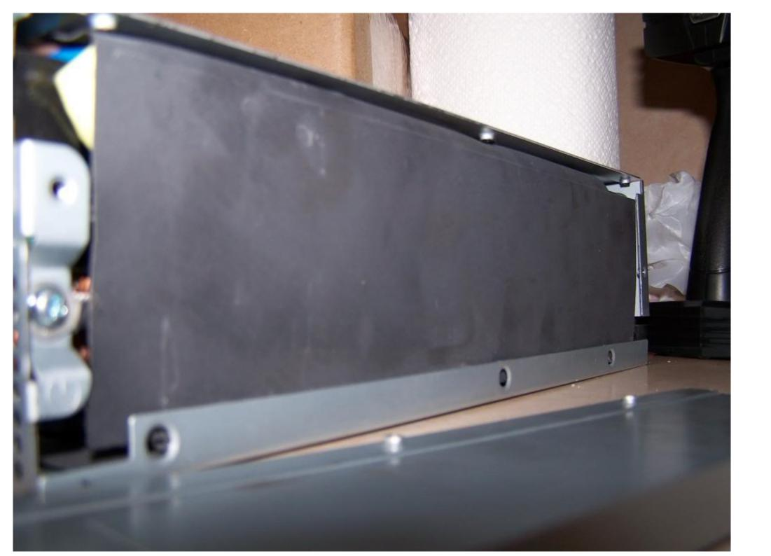
Now that the adhesive is broken, you should be able to slide the side panel apart like this. Then remove the fan screws.
