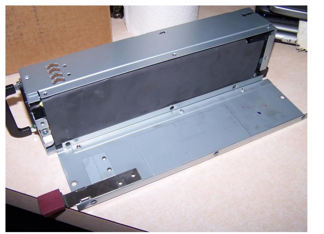
Using the top cover that you just removed as a knife, you're going to break the adhesive between the black insulation and the side panel at the top in this photo.
