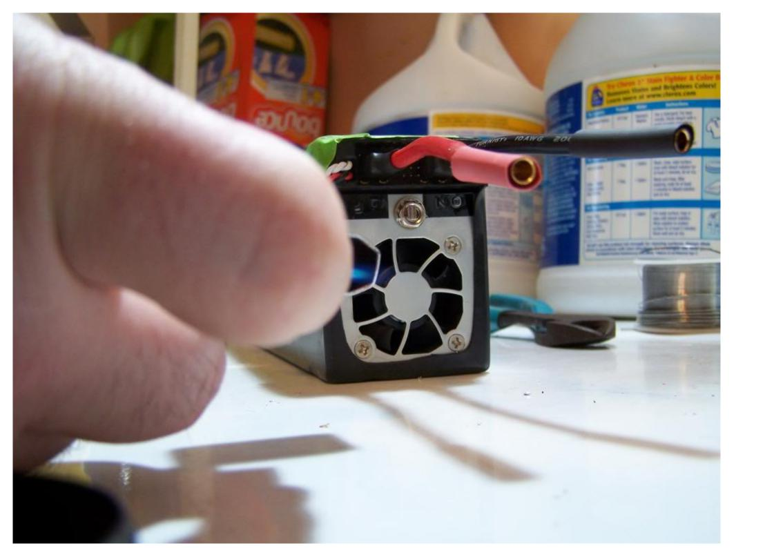
The very last step only applies if you are using two PSU in parallel like I did. You just need to take another jumper cable and connect pin 11 on both PSU together. That's it! Here's my finished setup:
