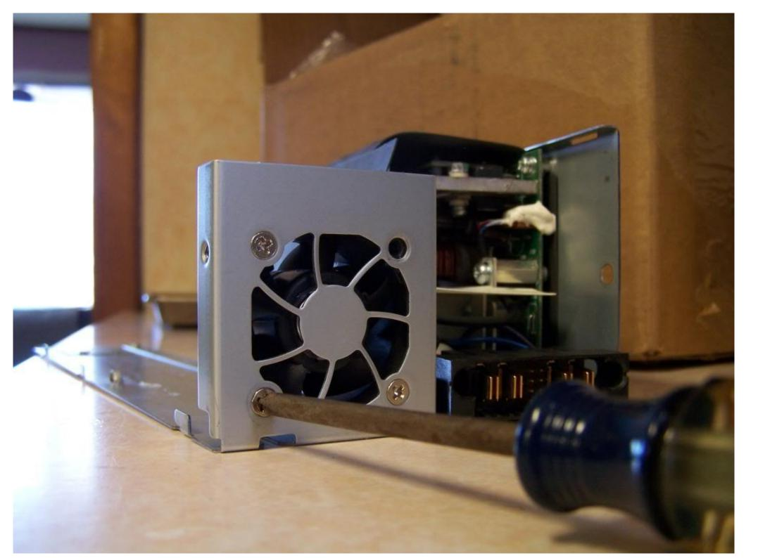
Once inside, you're going to want to isolate the DC ground in these two places. For the top arrow, I took that screw out, pried the board away from the standoff slightly, and placed 3 layers of electrical tape on the bottom side of the board. For the bottom arrow, you have to break those two connectors. It was pretty easy to do with needle nose pliers.
