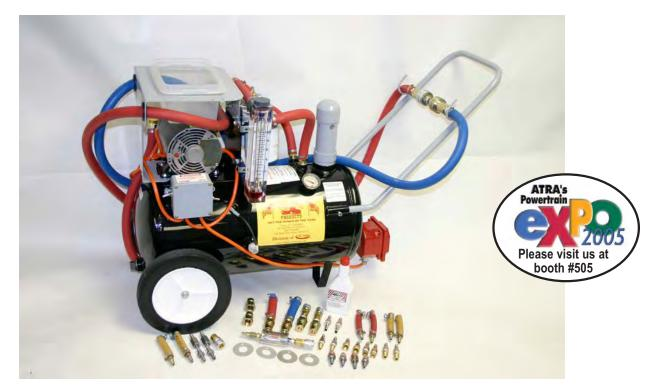
The <u>Heavy Duty Flusher</u> is the newest addition the to G-Tec line of heated cooler line flushers! It has all the features and benefits of the TTCF-7A Supreme Flusher (<u>www.g-tec.com</u>), however it utilizes 3/4" hoses, aircraft-style hydraulic couplings, 2" temperature gauge, 10 gpm flow meter, full 1 hp motor, and larger fittings to accommodate Allison® and International®-style transmissions.
