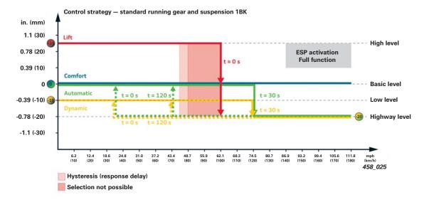
The control system enables four different vehicle height modes (levels). Starting from the basic level, lift mode can be set by raising the vehicle by 0.98 in (25 mm). Lift mode is immediately and automatically deactivated on reaching or exceeding a vehicle speed of 62.1 mph (100 km/h). This mode can be selected up to a speed of 50 mph (80 km/h).
