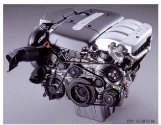
*Engine 611 With 2.2 I displacement and 60 kW to 95 kW used from 1998 to 2003 in C-Class, CLK-Class and E-Class.*
