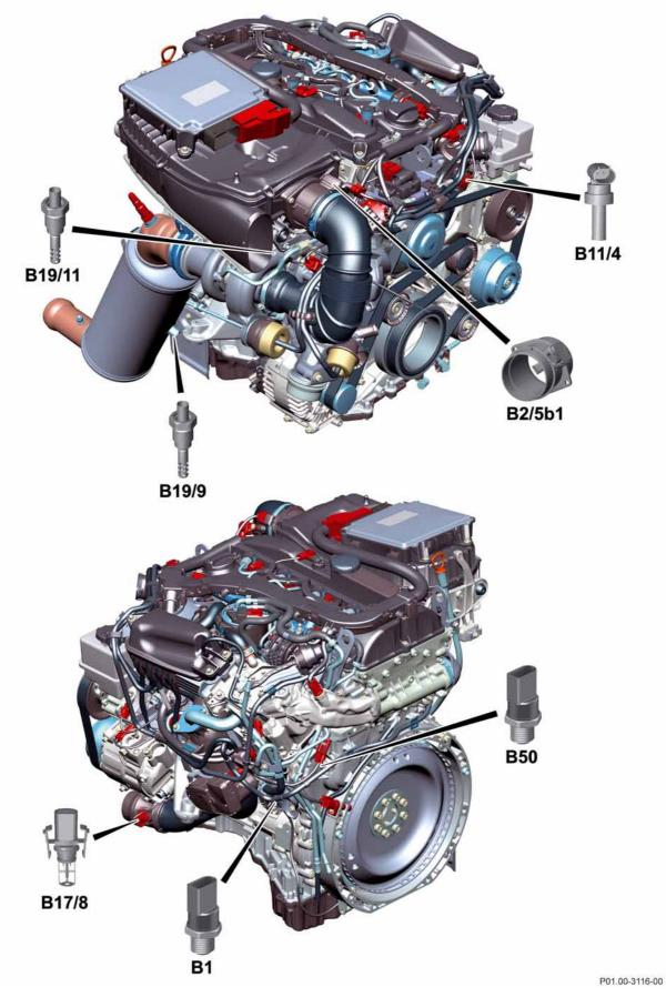
Engine 651 with temperature sensors
