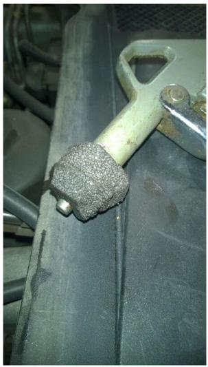
To avoid a mess inside the car, I fashioned a foam adapter to my air gun and applied air into the top pipe, while collecting the coolant into a ZipLock bag from the lower pipe. Be really gentle on the trigger, and do not close the zipper all the way, else you'll make a mess anyway. This was quite effective, not a single drop was spilled inside the car.
