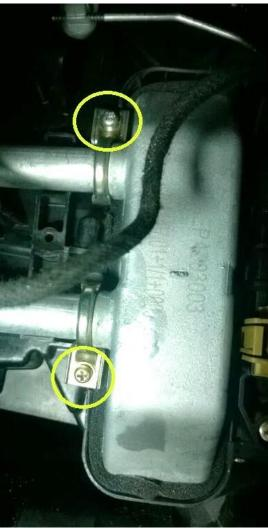
Disconnect the plug from the accelerator (grey cable on the above pictures). Remove the black plastic panel holding the core in place, two screws (Phillips). Loosen the clamps on the tubes into the core, again Phillips. Take a good look on how they sit; it's easy to put them back on just a little bit off. When it sits right, it's easy to pinch it all the way shut with two fingers.
