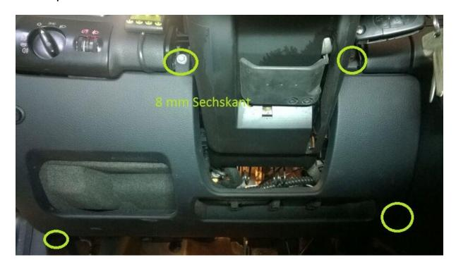
Remove the little panel above the steering column. It slides backwards, away from the instrument cluster. Unscrew the under dash panel, 4 bolts (8 mm hex). Unclip the OBDII-connector from the panel. Disconnect wires from the foot well light. Lift out panel.
