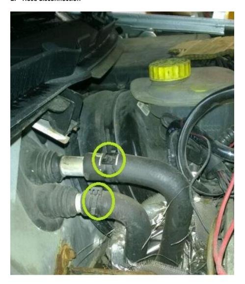
Use clamp pliers or general purpose pliers to loosen the clamps and slide them back along the hoses. If you have hose clamps, now is a good time to clamp off the hoses, if not, you'll lose about a litre of coolant. Or stuff something into the hose openings afterwards. Slide the hoses off the pipes. Be careful, those pipes are made of aluminium foil and dents very easily.
