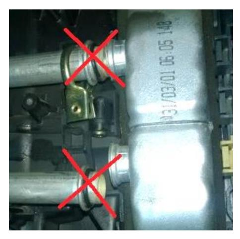
From that position, it doesn't seem to be possible to make them enter the recesses in the core housing properly, and it is not possible to get the clamps to fit over the respective ridges.
