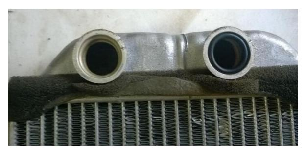
Now the pipe ends must be precisely positioned over the holes, then eased in through the rings. This is where it gets interesting. The tiniest little skewness makes the O-ring pop out on one side or get drawn into the core on the other side. Both the core and the pipes will have to be wiggled a bit about to make them mate properly.
