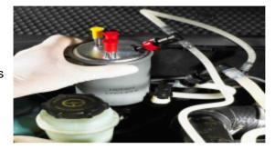
If the pressure can be recovered by a new IMV proceed to the next step. The injector back leakage is critical and must be within the parameters outlined in the test kit manual. If the back leakage is not uniform between the cylinders then the highest back leak injectors
