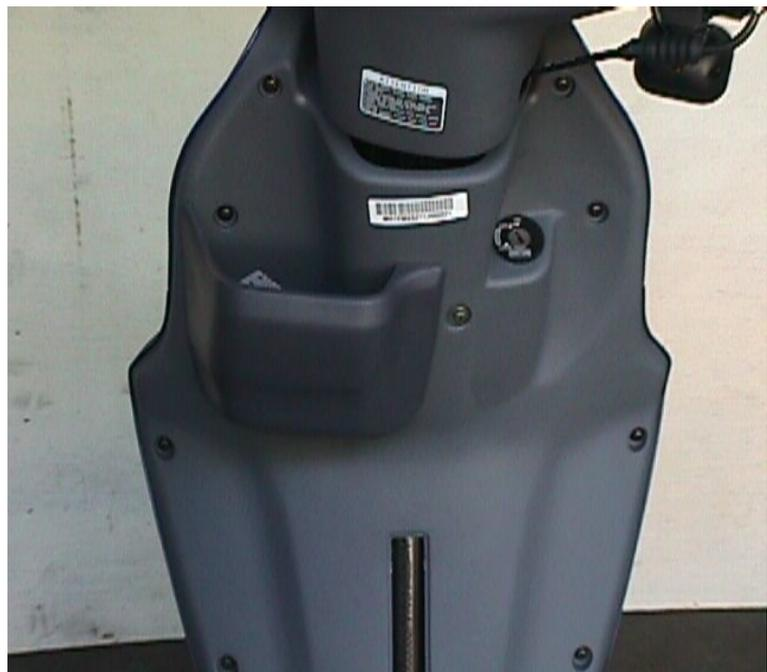
11.screwing out the screws of front mudguard.
