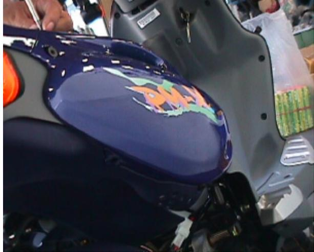
8.Screwing out the screws of rear cover
