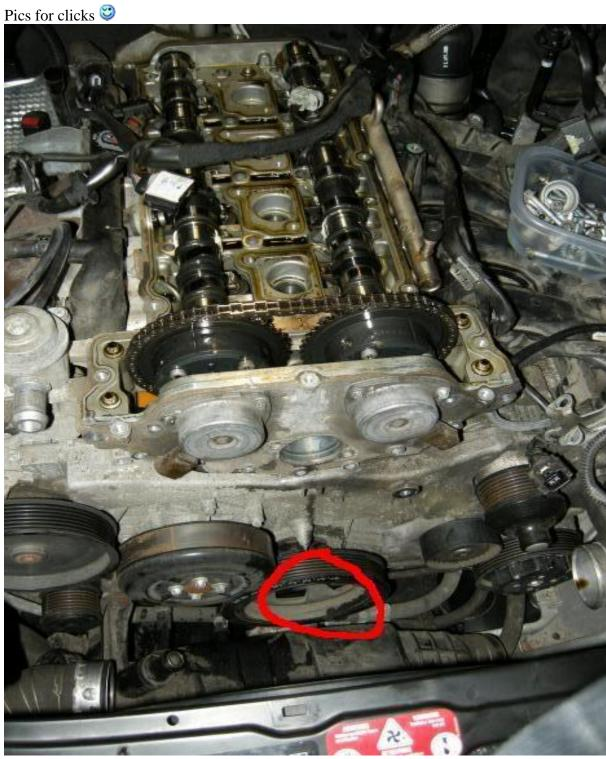
incase anyone ever finds this thread, it is 'normal' or counter clockwise to loosen it. And it requires like 170ft/lbs of torque.
