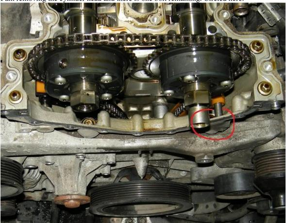
The 'slide rail pin' that holds the driver-side chain tensioner is in the way of getting a socket on it. Looks like i need some kind of \$150 116 589 20 33 00 Impact Puller for slide rail bearing bolt, basic unit. <a href="http://www.samstagsales.com/SirTool/...ompleteset.jpg">http://www.samstagsales.com/SirTool/...ompleteset.jpg</a>
