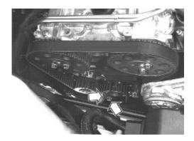
Check that there is no visible leakage. Compress the tensioner damping unit with tool <u>999 5456</u>. Position tensioner damping unit in the tool and screw tool center nut to the bottom. Wait until compression is complete and install a **2 mm** lock pin in the piston.
