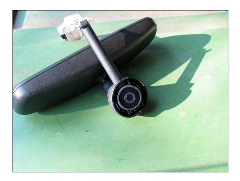
Make a note of the white bundle attached to the top of the mast that hides the wires. This routes all the wires and mounts the wires to the inner roof of your car. There is a better shot of it in these dissection pictures - one from far away and a closeup:
