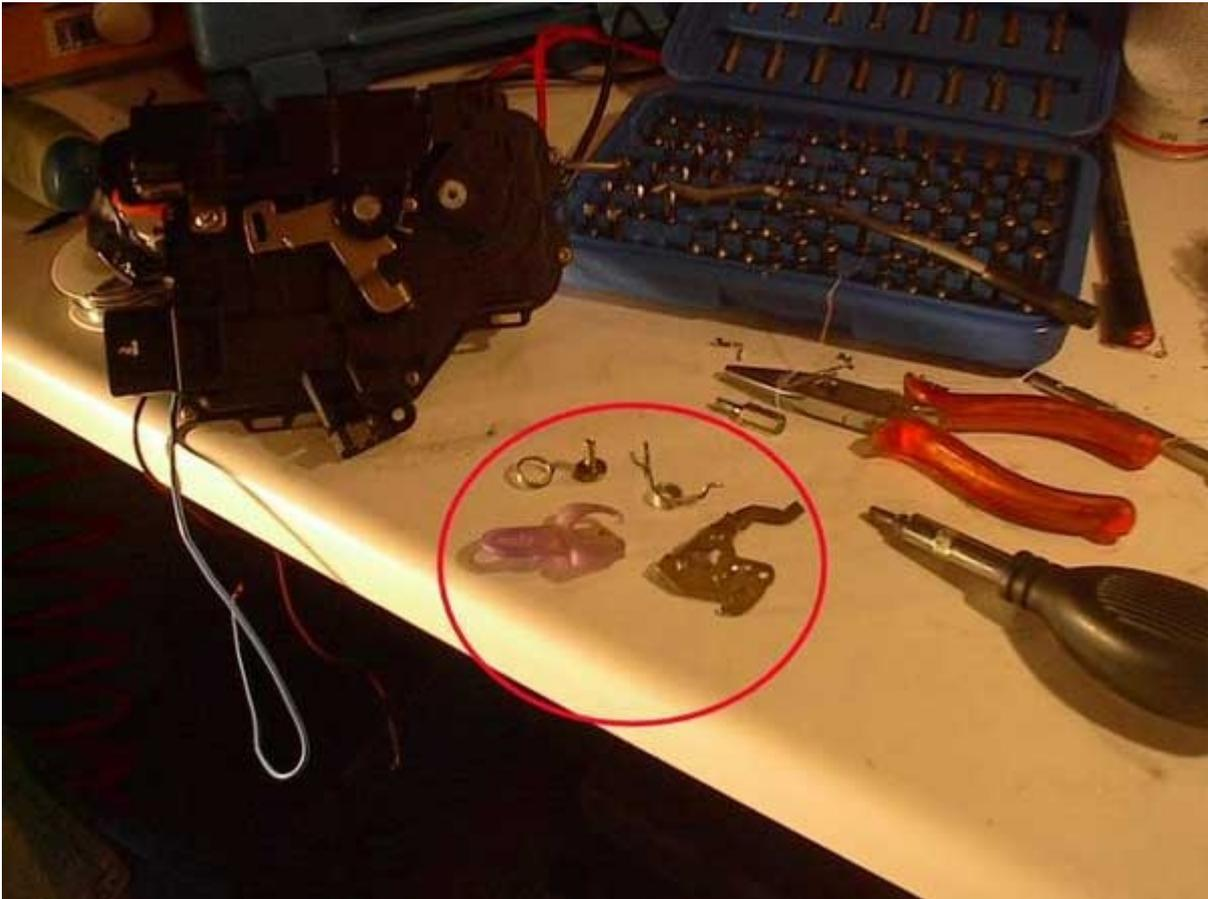
The four parts left after you've put the two main parts together (all the torx)
