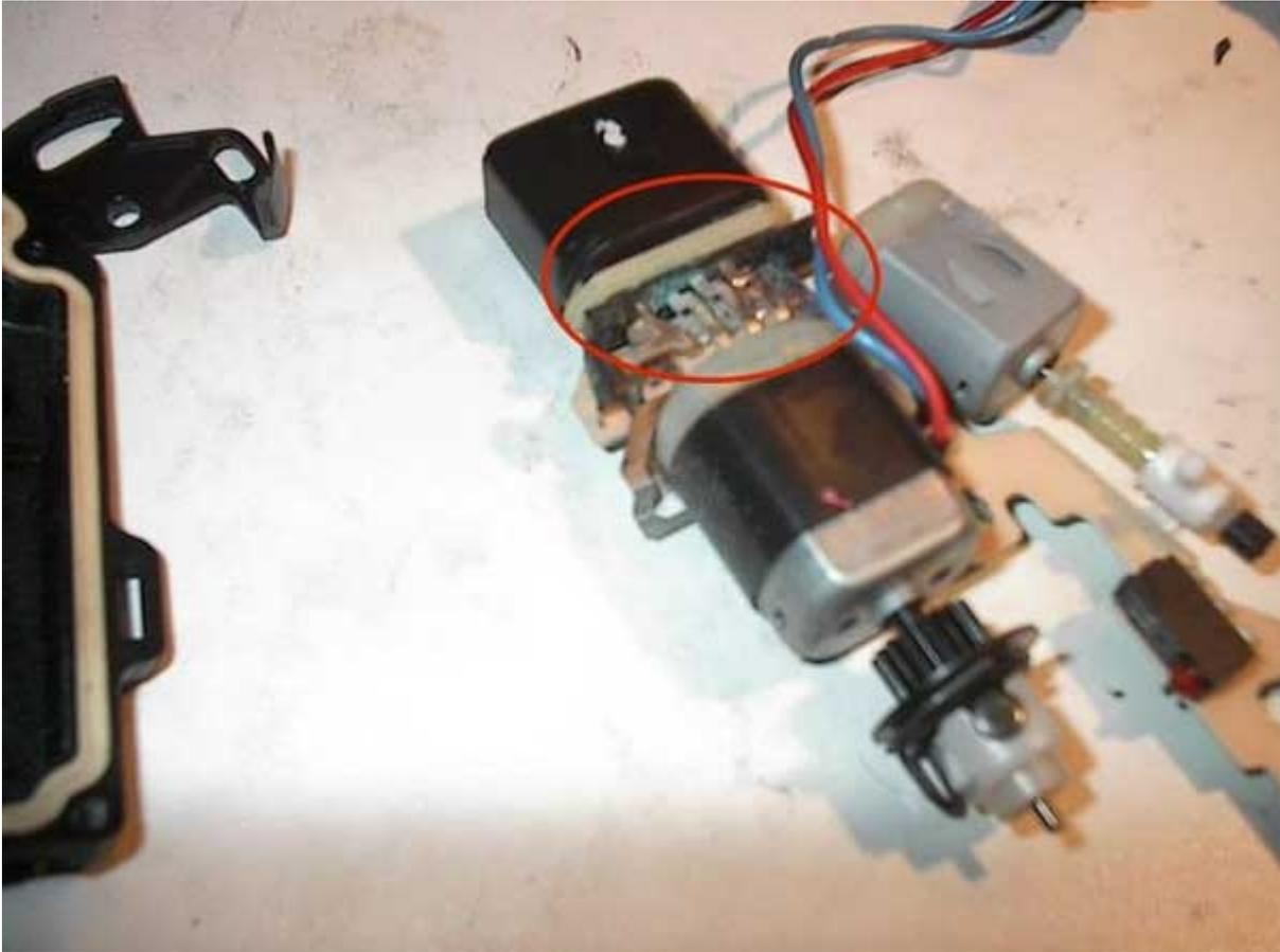
Ugh.. bad pic, but you see the corrosion. When the latch is installed, this is the absolute bottom of the box - and when the box is not tight, water/damp concentrates here..
