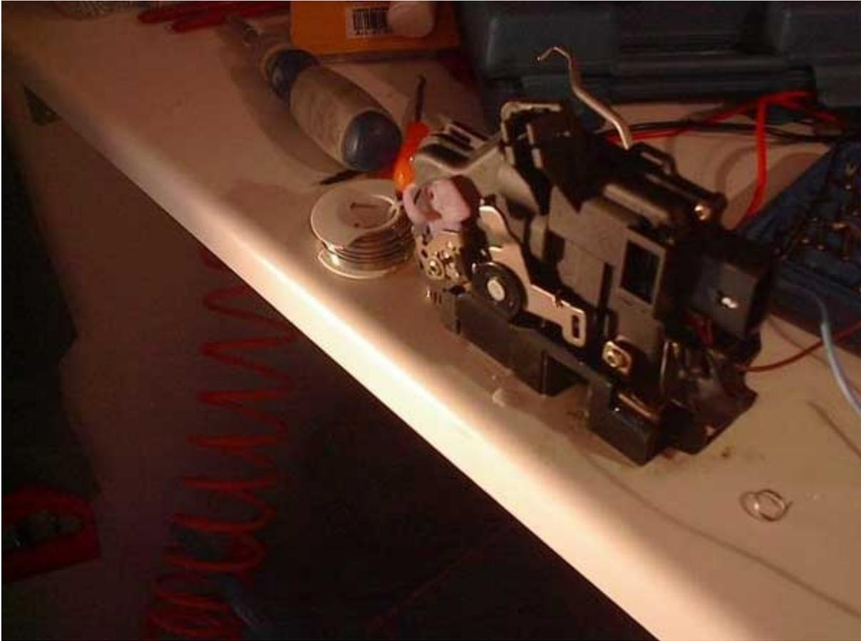
You'll have to wiggle a a bit to get this arm right, and I had to set the torx screw just inside, so I could pull out the white rod that the metallic/plastic arms are connected to. You'll figure it out! Don't screw tight before you see that the white rod are lined up with the white arm.
