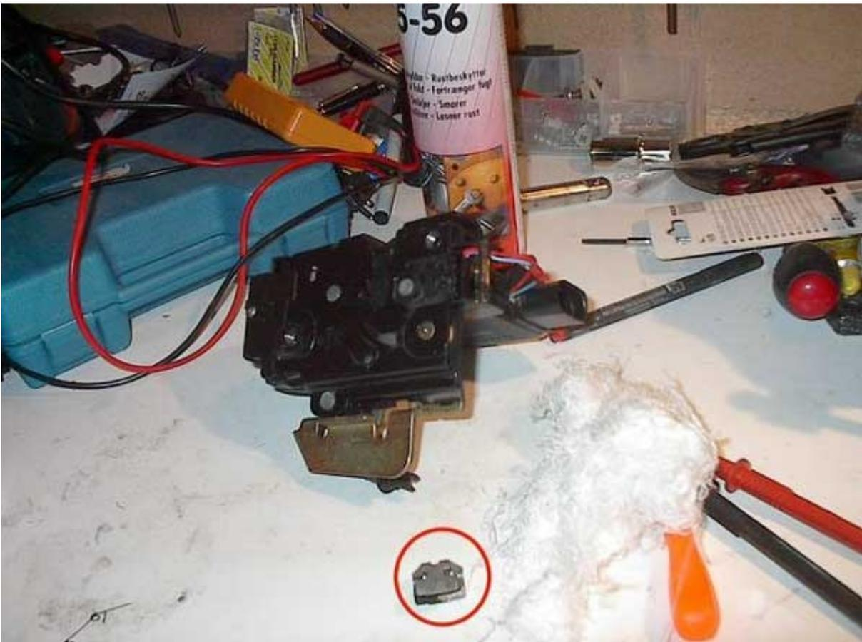
The red ring shows the metallic clamp that holds the sensor to the latch. Just flips off.
