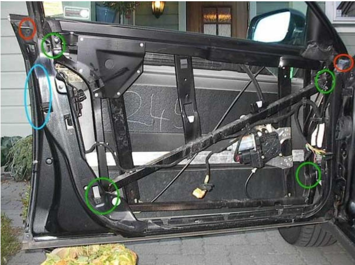
The blue rings shows two M8 screws that actually holds the latch. Flip off the plastic that hold the lock rod. Pull that rod off. Then the key rod. You'll have to wiggle that out (pull a bit down and turn clockwise, it just holds by the rods length).
