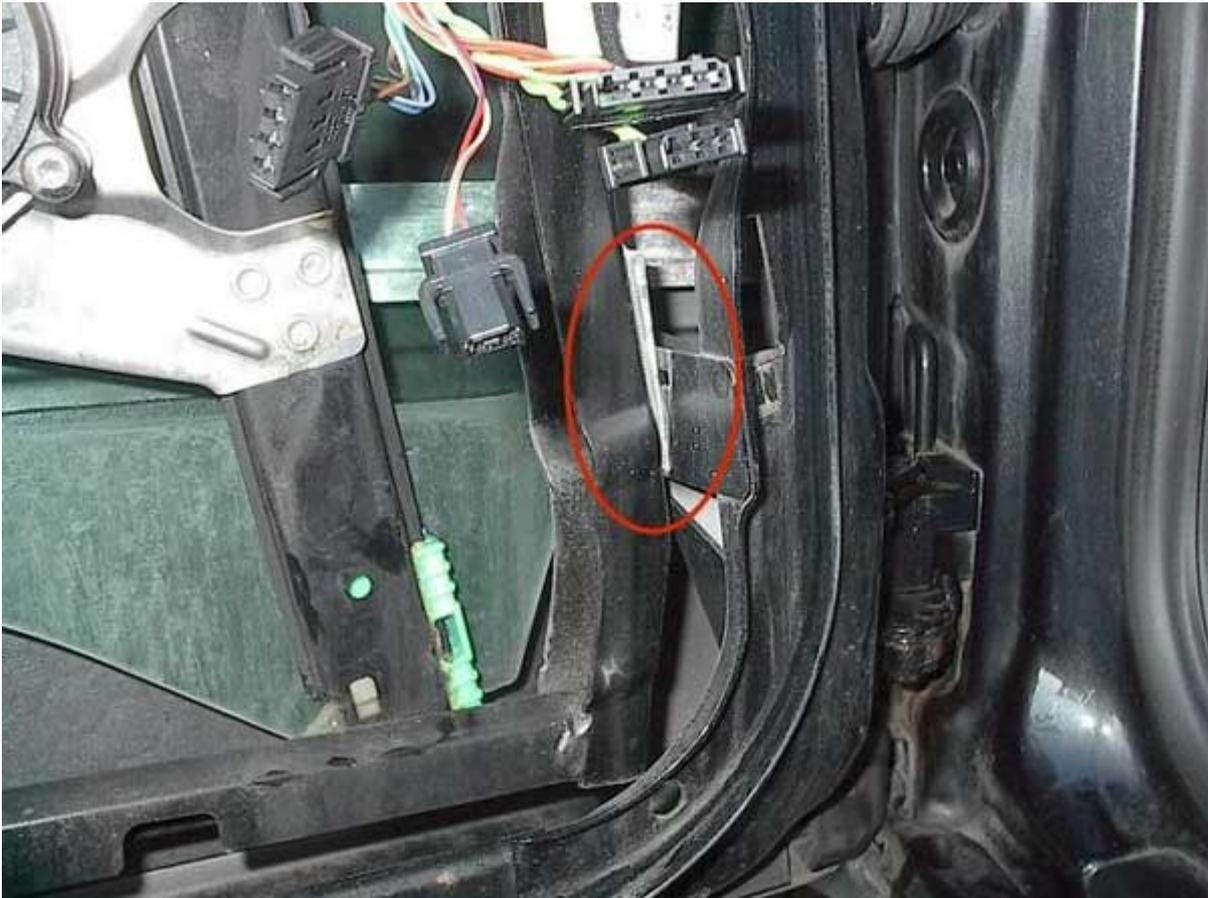
I took off the window mount, just because I got more room. Remember how it was mounted.. Would be easier to remount. The prev pic showed 4 green rings. Torx 45. When remounting, you should fasten the upper two before the torx on the bottom (work right to left)
