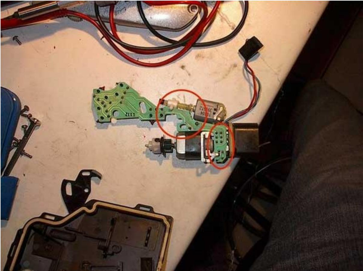
Here's the circuit board. The rings shows where most of the corrosion where. On the thin electric lines and down by the connector (on the other side - se pic below).
