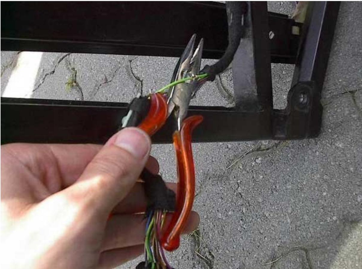
Reattach the latch and hot-wire the new connectors you made into the wires from the car. For my experience, I had to make new connectors for line 4 and 6.
