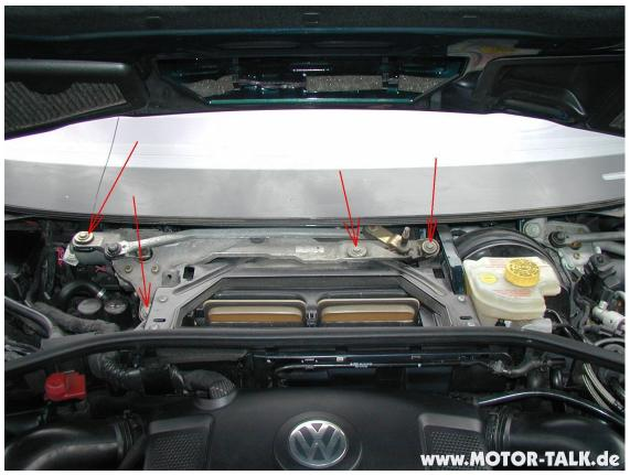
The photo below shows the left hand (driver side in NAR) assembly in situ before removal. It is not particularly difficult or time-consuming to remove this assembly, however, like all other Phaeton repairs, you need to pay attention to what you are doing because the car is rather complex, and you run the risk of screwing up something else totally unrelated to the system you are working on if you don't put everything back together properly.
