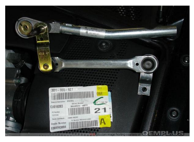
7) To actually get the assembly out of the car, you only have to remove three bolts. This is pretty easy, as you can see from the photo below.
