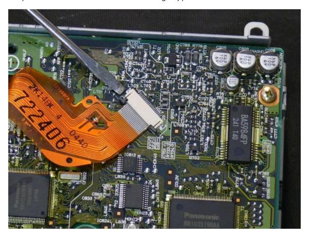
Here we have the second ribbon connector. This picture shows the ribbon clamp more clearly. It is in the "out" position ready for the ribbon cable to be removed.
