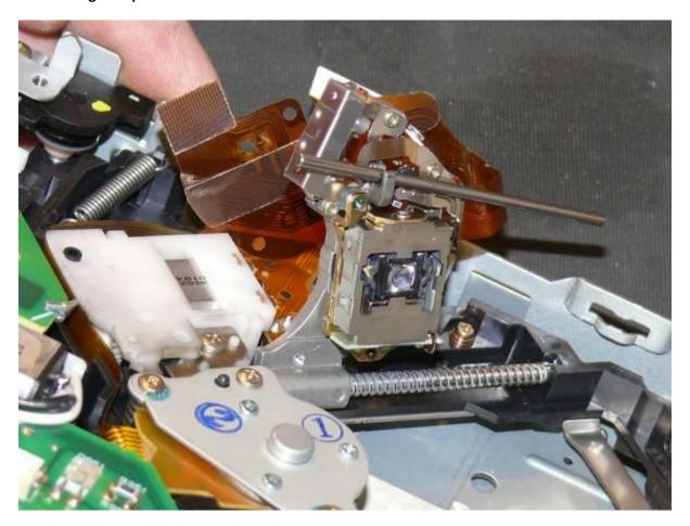
This screw holds the motor mount for the laser light. The picture clearly shows the worm drive that moves the laser light radially across the DVD.
