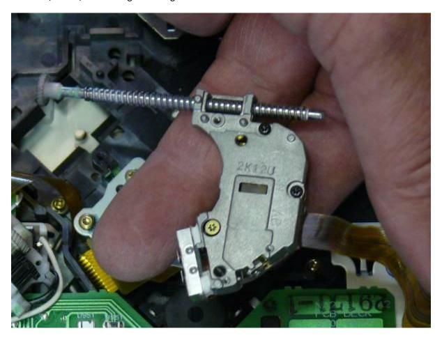
Just for the record, and to show the numbers, here are the two laser units, old and new. I have already fitted the worm gear to the new laser unit.
