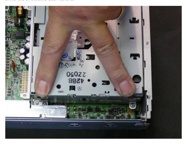
Removing the screws holding the DVD mechanism. A pair of tweezers can be useful here.
