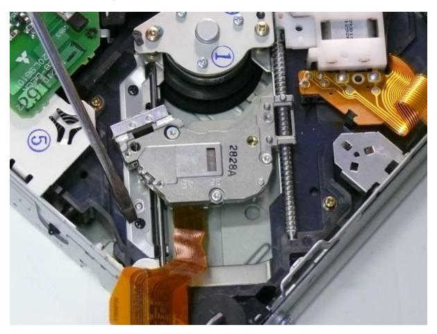
Here the retaining clip for the laser unit guide bar is being removed.
