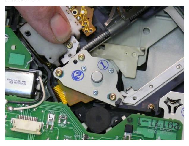
Carefully prise the motor unit from the chassis. The clips are difficult to see. I have indicated their position in the photograph.
