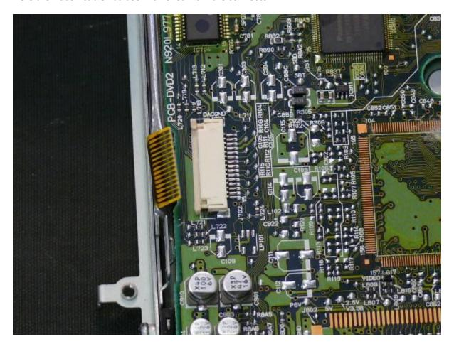
These screws hold the CB to the chassis. They must be removed.
