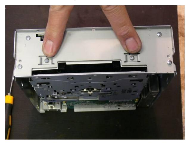
Remove these four screws. Two either side of the connectors.
