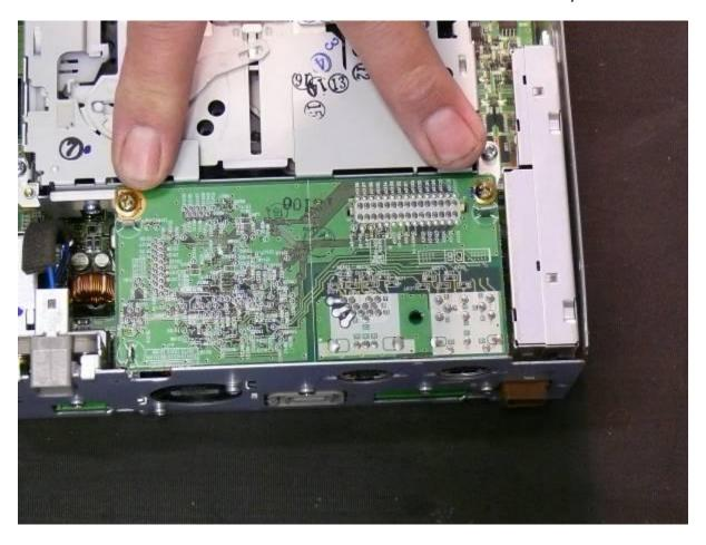
Check these tabs. Mine were twisted to hold the CB. If necessary twist gently to align with the slots in the CB.
