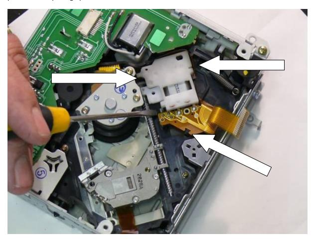
Prise out the motor mount (care required). Note that it is still connected via a ribbon cable that I did not remove. Just gently put the motor to one side.
