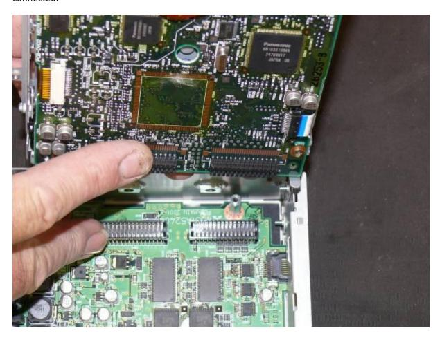
This cable has the clamp mounted on the underside of the CB, hence the CB needs to be "hinged" up to gain access to the ribbon connector – visible at the end of my finger. Remove the clamp using the same process as before. Remove the cable.
