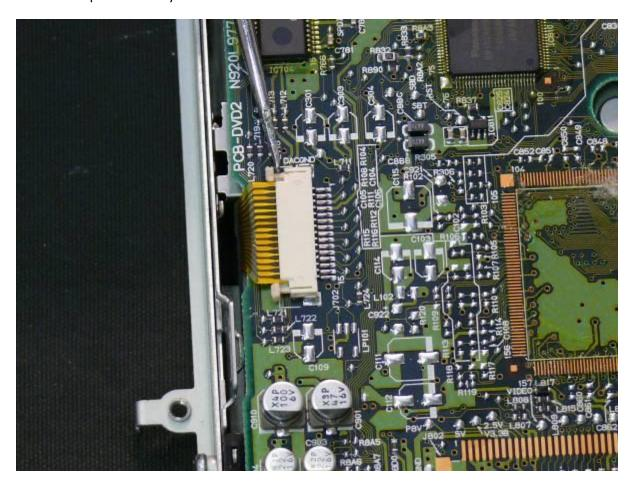
Here the ribbon cable has been removed from the connector.
