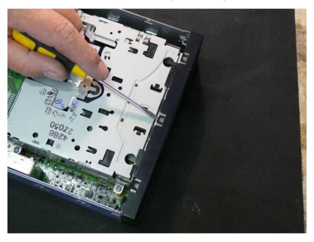
Note the small connector that connects the front cover to the chassis.
