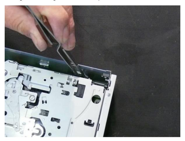
After removal of the 4 screws the DVD drive mechanism can be prsied form te chassis. There are 2 connector blocks which will unplug as you remove the mechanism. See later photograph for a view of the connector blocks.
