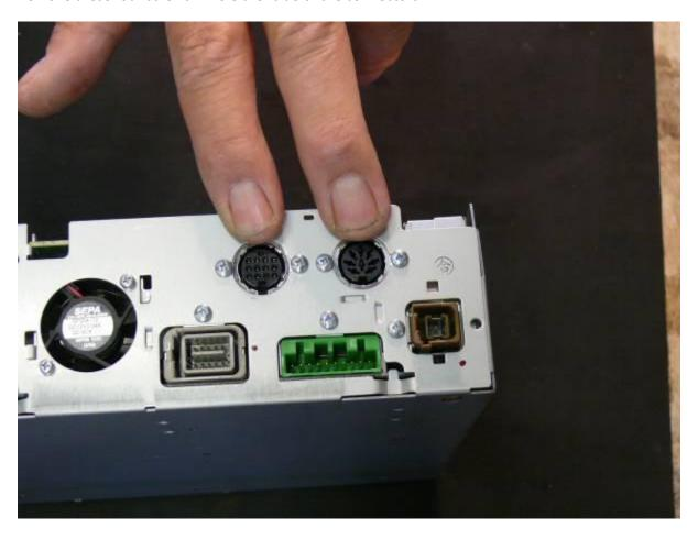
Remove these screws that hold the circuit board to the chassis. Do not remove CB yet!
