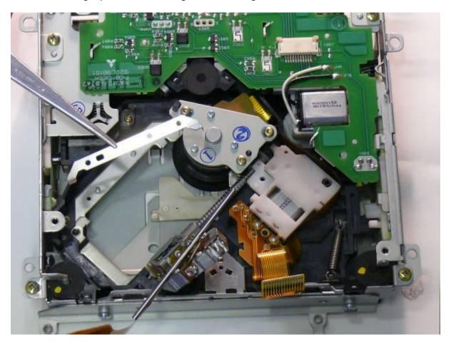
Here the laser has been lifted. The arrangement for the slide bar can be clearly seen. This picture also shows the laser light itself. If the aim is to clean the light – this can be done now, no further dismantling is required.
