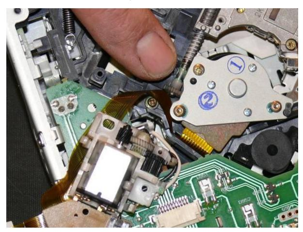
And here, at last, the laser light is being lifted from the drive.
