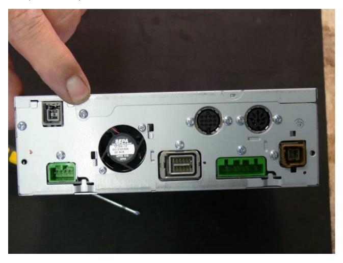
These notches can be used to prise the top cover off. Use a flat bladed screwdriver and twist – gently.
