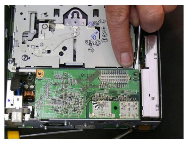
Here you can see the CB being removed. Note the plug connector that connects the CB to the "motherboard".
