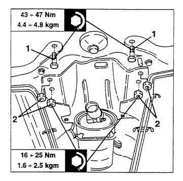
1. Slacken the fastening screws and remove the power unit rear support.
