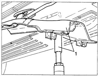
1. Disconnect the gearshift control lod from the lever slackening the fastening bolt.
