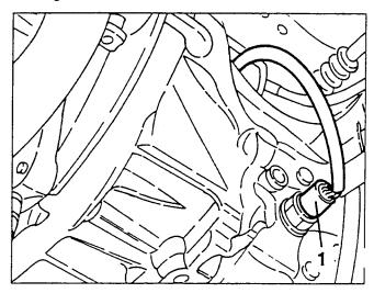
1. Disconnect the electrical connection of the lambda sensor.
