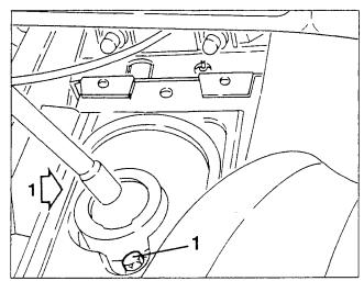
1. From under the car, retrieve the gearshift control lever complete with joint and frame.
