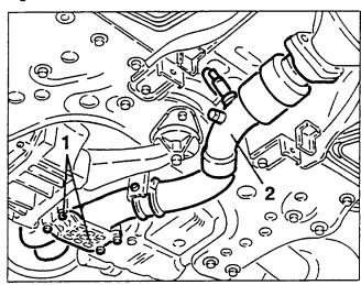
1. Slacken the bolts fastening the wishbones to the wheel uprights.
