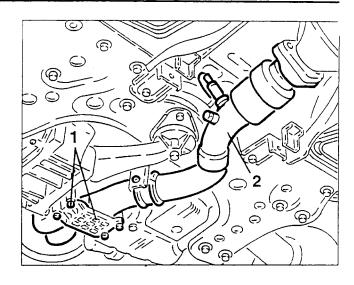
1. Slacken the fastening bolts and remove the catalytic converter complete with the first silencer of the exhaust system.
