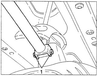
1. Disconnect the gearshift control rod from the support on the power steering box slackening the fastening nut.
