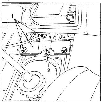
Disconnect the electrical connection of the lambda sensor.
