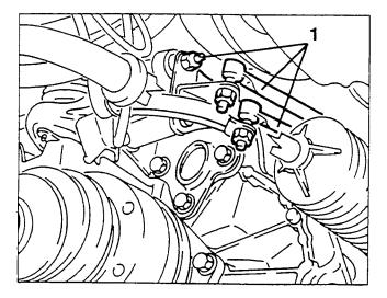
1. Slacken the three screws fastening the starter motor to the gearbox.
