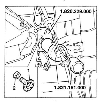
1. Using tools no. 1.821.170.000 and no.1.821.171.000 install the new oil seal.
