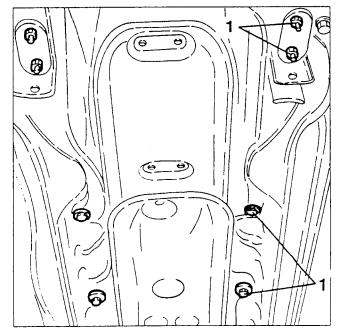
1. Using a hydraulic jack as support, lower the front of the gearshift controls support as illustrated.
