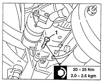
1. Slacken the fastening screws and bolts and remove the gearbox side power unit support.
