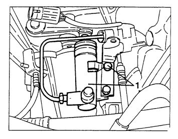
1. Disconnect the electrical connection from the reversing switch.
