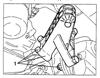
1. Slacken the two lower screws fastening the gear-box cover and in their holes insert bracket no. 1.820.623.001.
