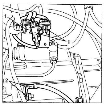
1. Slacken the fastening screws, then move aside the clutch control cylinder without disconnecting the hoses.
