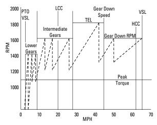
Note how Lower Gears and Intermediate Gears setting fit in the total spec, especially in respect to Top Engine Limiting (stair step effect).
