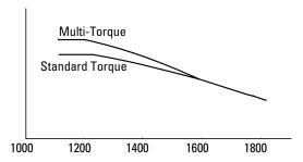
The ECM determines when the vehicle is in the top gears by calculating the ratio of engine speed to vehicle speed. If the ratio is greater than 71.5, the engine will operate with the standard torque curve.
