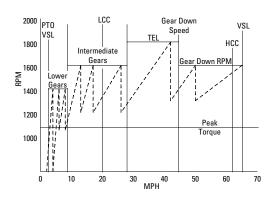
It is important to note that although Low/Intermediate Gears parameters are "soft" limits, Gear Down Protection is actually a "hard" limit.
