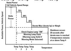
As Coolant temperature rises to 217°F (103°C) the engine is derated by 25% of the Delta Hp. In this example 240 Hp x .25 = 60 Hp. The driver would have 340 Hp available. If the driver reacted by downshifting, for example, and the temperature did not rise, the power would stay at this level.
