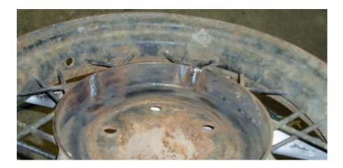
The wheels should be cleaned and preferably the paint removed from them along with the rim liner. The spokes will be heated and the resulting fumes from burning paint can't be the best for your health. Clean wheels will also be easier to work with.
