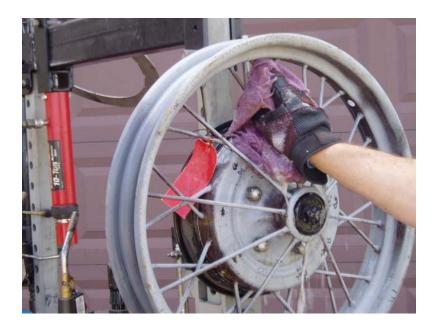
THE RAG IS SURROUNDING THE SPOKE AND QUICKLY MOVED UP AND DOWN THE LENGTH OF THE SPOKE UNTIL THE SPOKE IS COOLED. THE PROCESS IS REPEATED AS OFTEN AS NECESSARY TO PROVIDE THE CORRECTION DESIRED. IT MAY BE NECESSARY TO HEAT TWO OR THREE CONSECUTIVE SPOKES TO ACHIEVE A LARGE AREA CORECTION. THE PROCESS IS THE SAME FOR ALL YEARS OF MODEL A WHEELS.
