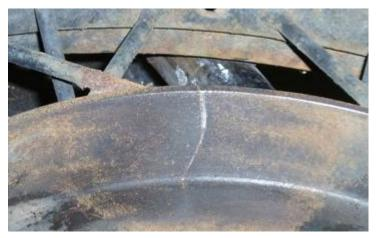
Check for cracks in the hub area.
