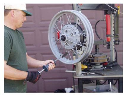
STRAIGHTEN ALL BENT SPOKES. I AM USING THE SPOKE STRAIGHTENING STATION ON MY HYDRALIC PRESS TO DEMONSTRATE THE PROCESS BUT YOU WILL BE USING THE FRONT AXLE OF YOUR CAR TO COMPLETE MOST OF THE OPPERATIONS OF SPOKE STRAIGHTENING. (The photo above was staged for the development of this document. Note that safety glasses are missing and should be worn.)
