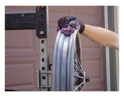
COOL THE OUTER AREA OF THE RIM FIRST BY HOLDING THE WET RAG ON THE AREA PREVIOUSLY HEATED UNTIL THE SIZZLING STOPS AND THEN QUICKLY MOVE TO THE SPOKE AS SHOWN IN THE NEXT PICTURE.
