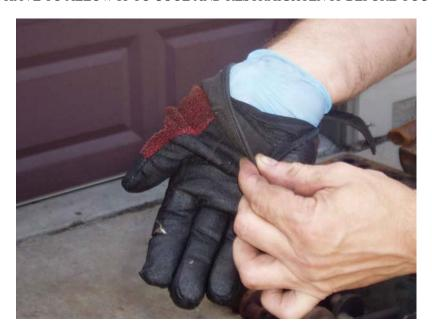
THE SPOKES NEED TO BE QUICKLY COOLED TO CAUSE THE "SHRINK" OF THE SPOKE. THE SPOKE AND RIM WILL BE VERY HOT AND STEAM WILL DEVELOP DURING THE PROCESS. I USE A NITRILE GLOVE INSIDE A DURABLE MECHANIC'S GLOVE TO PROTECT MY HAND FROM THE STEAM.
