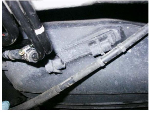
\*STEP 3\* Using a pry bar or something like it GENTLY pry the front of the gas tank down enough to slip a 2x4 up and kind of on top of the tank. this will hold the tank in the downward position.
